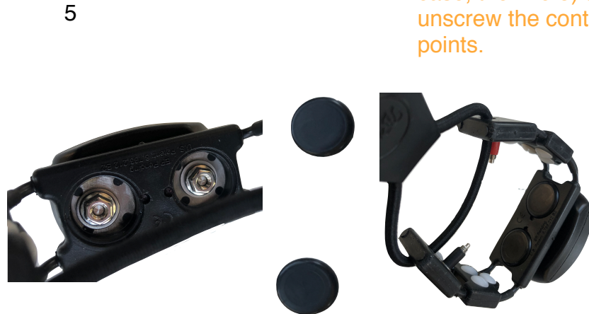
5 Tighten the washers and bolts, and then replace the covers on the back of the CEMS®.
