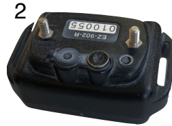
2 Take my receiver that is compatible with the Chameleon® Extender and unscrew the contact points
