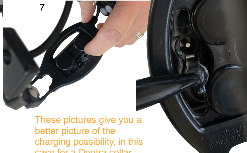
4 Place the receiver such that the posts for the contacts fit through the holes in the center piece of the Extender with the posts of the receiver facing to the inside of the Chameleon® Extender.
